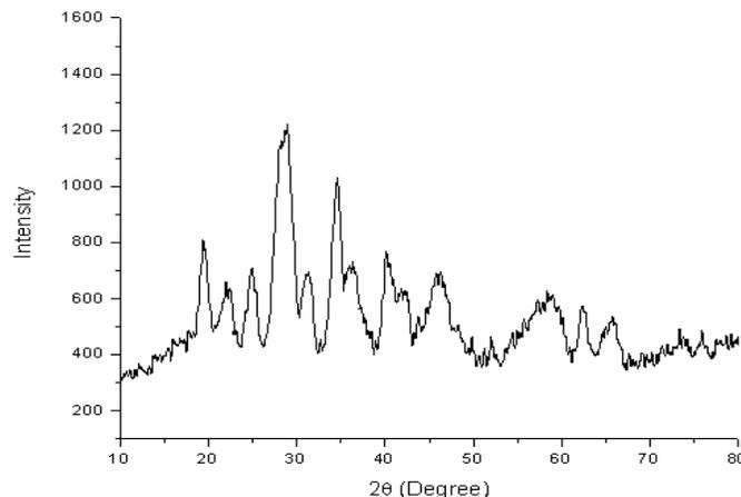
Fig. 2 X-ray diffraction pattern of SrAl<sub>2</sub>O<sub>4</sub>: Eu, Dy phosphor
