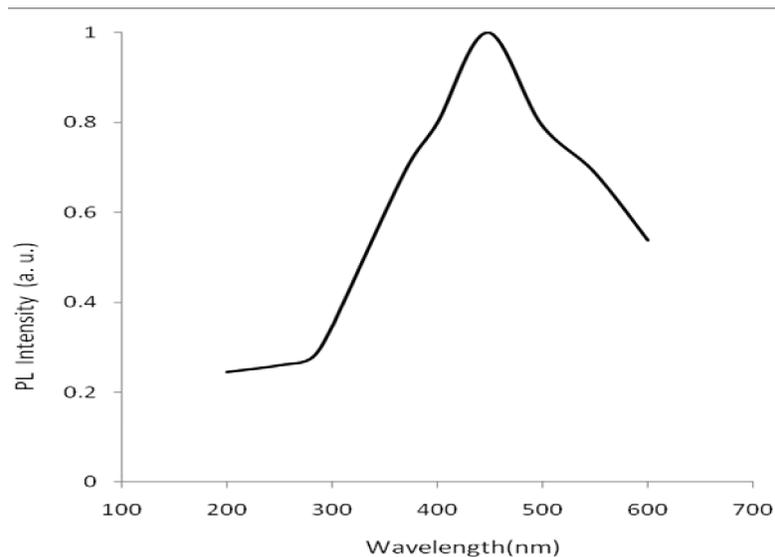
Fig. 3 PL emission spectra of  $\text{SrAl}_2\text{O}_4$  phosphor
