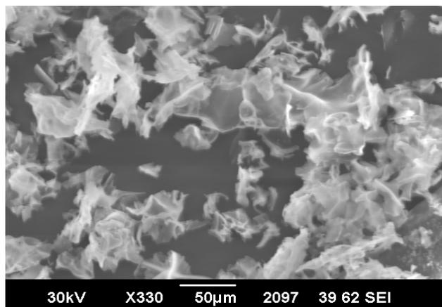
Fig. 1 SEM micrographs of SrAl<sub>2</sub>O<sub>4</sub>: Eu, Dy phosphor
