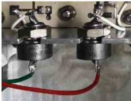
**Figure 3.** Feed-through for DC power supply
