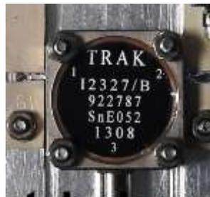
**Figure 1.** Isolator in the circuit
