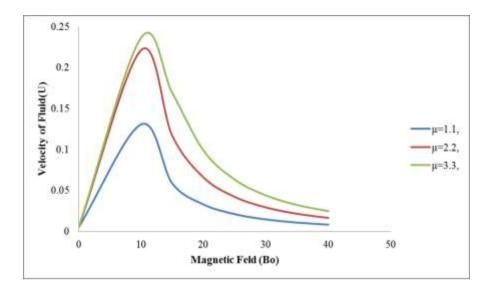
The graph shows that the velocity profile of fluid with respect to magnetic field for different values of fluid viscosity as magnetic field increases, velocities also increase from the values nearly equal to zero and take a maximum value around M = 10, and then decreases sharply following a resonance character.
