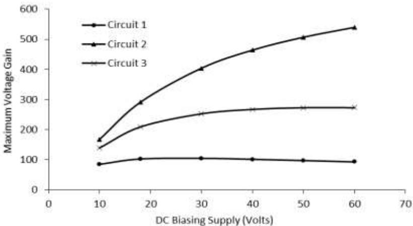
**Figure 3.** Variation of voltage gain with DC biasing supply
