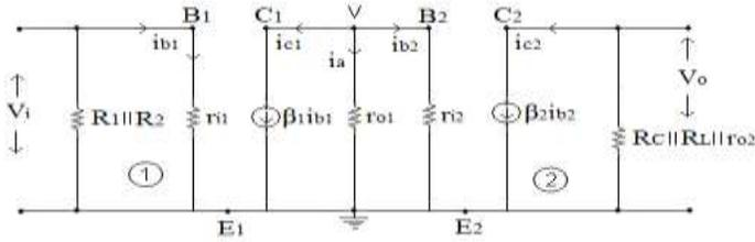
**Figure 4(b).** Reduced AC equivalent circuit corresponding to the proposed amplifiers
