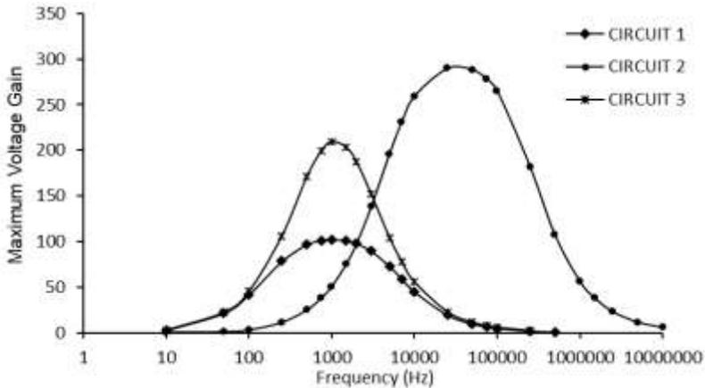
**Figure 2.** Variation of Voltage gain with frequency for reference and proposed amplifiers
