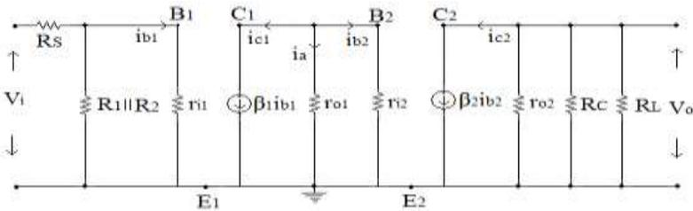
**Figure 4(a).** Small signal AC equivalent circuit corresponding to proposed amplifiers
