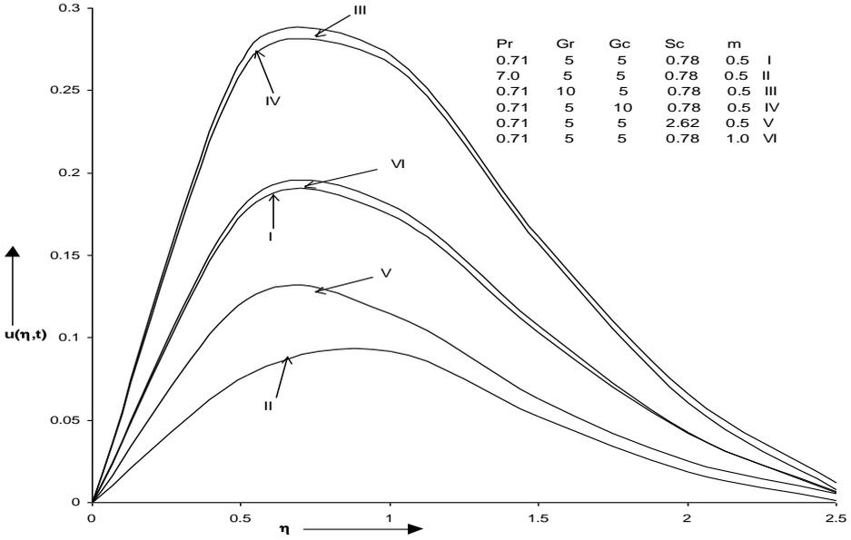
Fig.2. Axial velocity distribution versus  $\eta$  when  $N=1, M=1, K=1, \omega=10, \omega t=\pi/6$  and  $S=-1$ .
