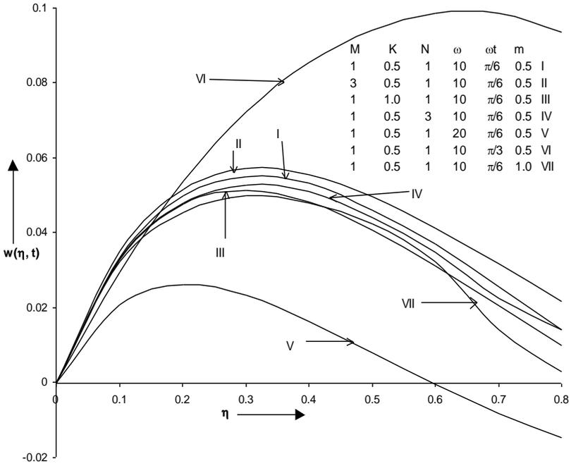
Fig.8. Normal velocity distribution versus  $\eta$  when  $Pr = 7.0$ ,  $Gr = 5$ ,  $Gc = 5$ ,  $Sc = 0.78$  and  $S = -1$ .
