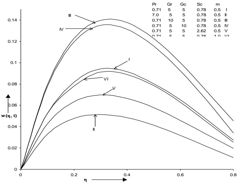
Fig.6. Normal velocity distribution versus  $\eta$  when  $N=1, M=1, K=1, \omega=10, \omega t = \pi/6$  and  $S=-1$ .
