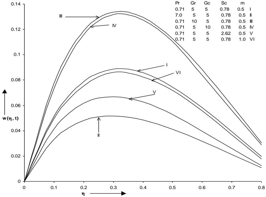
Fig.5 Normal velocity distribution versus  $\eta$  when  $N=1, M=1, K=1, \omega=10, \omega t = \pi/6$  and  $S=1$ .
