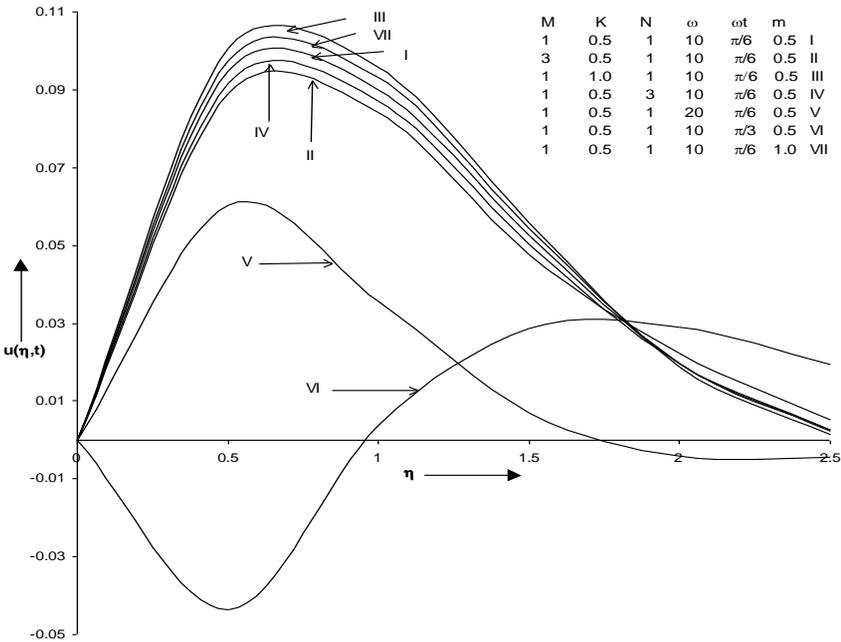
Fig.3. Axial velocity distribution versus  $\eta$  when  $Pr=7.0, Gr=5, Gc=5, Sc=0.78$  and  $S=1$ .
