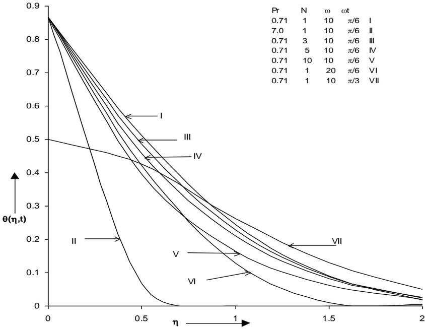
Fig.9. Temperature distribution versus  $\eta$  when  $S = 1$ .
