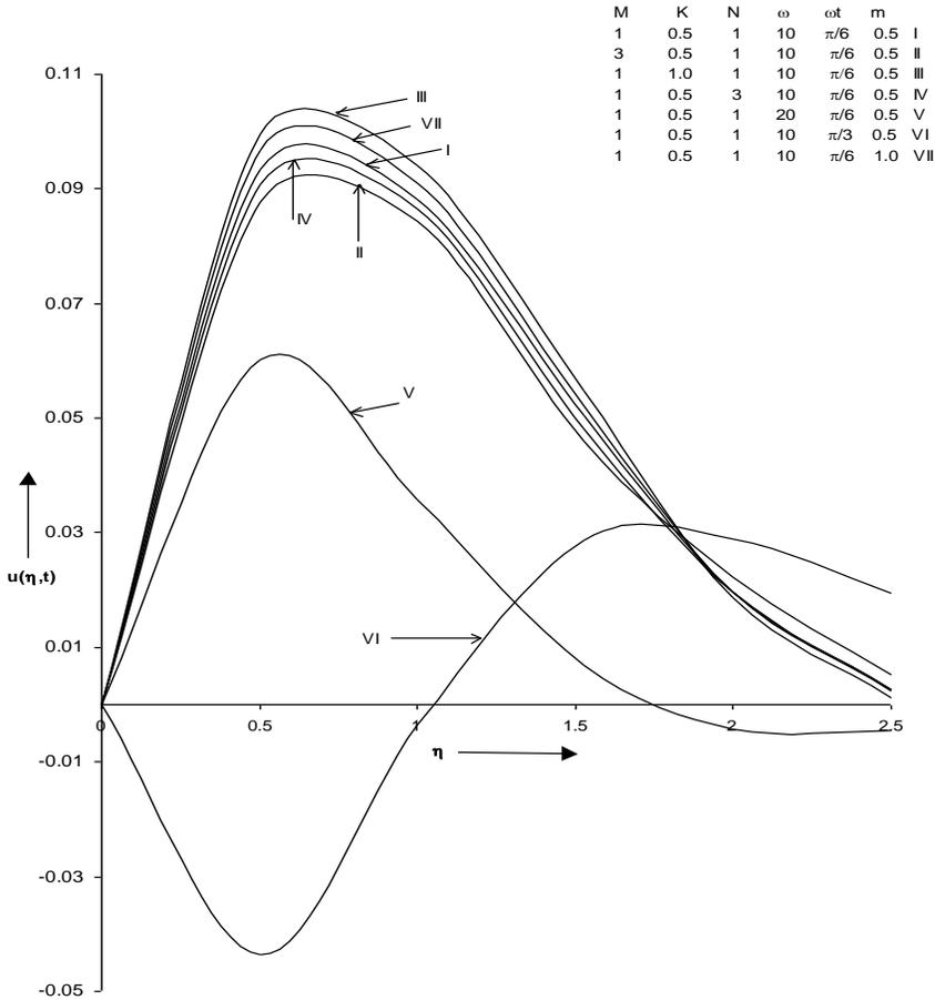
Fig.4. Axial velocity distribution versus  $\eta$  when  $Pr = 7.0$ ,  $Gr = 5$ ,  $Gc = 5$ ,  $Sc = 0.78$  and  $S = -1$ .
