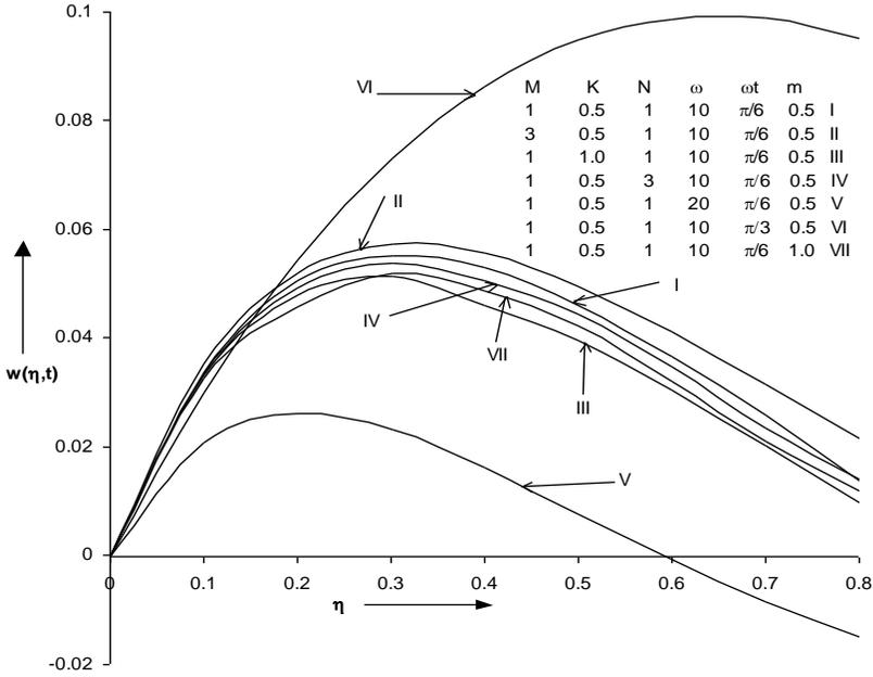
Fig.7. Normal velocity distribution versus  $\eta$  when  $Pr = 7.0$ ,  $Gr = 5$ ,  $Gc = 5$ ,  $Sc = 0.78$  and  $S = 1$ .
