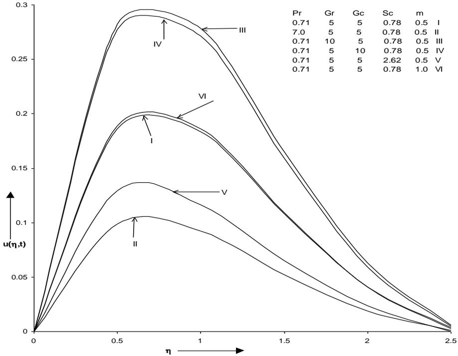
Fig.1. Axial velocity distribution versus  $\eta$  when  $N = 1, M = 1, K = 1, \omega = 10, \omega t = \pi/6$  and  $S = 1$ .
