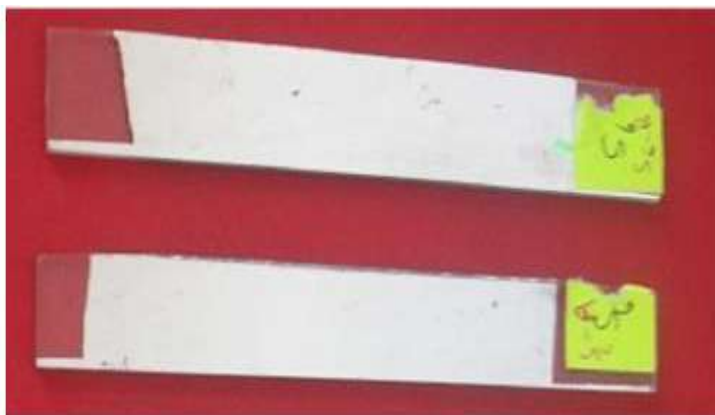
Figure 10. Transparent parts indicate glass substrates and white parts indicate coated Al thin films.
