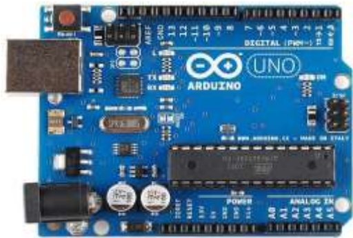
Figure 3. Arduino UNO used in the system
