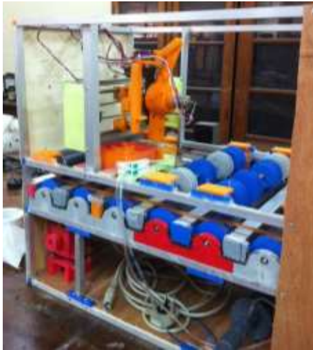
Figure 1. Designed roller converter
