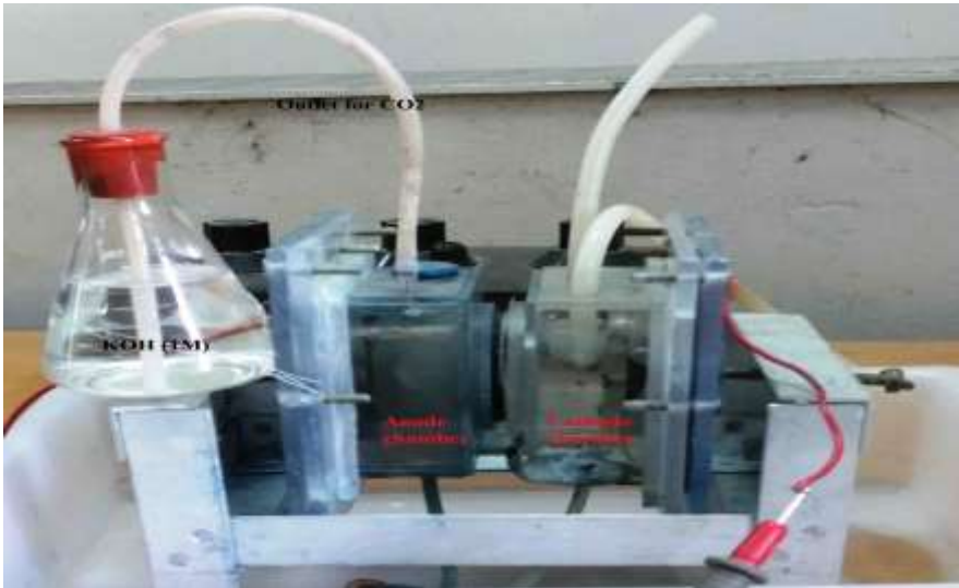
Figure 1. MFC with arrangement for CO 2 trapping
